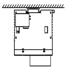
Where the ambient temperature will not exceed 35°C (95°F), the compact bases may also be mounted upright on a horizontal plane as shown below:
