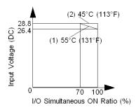
Also, when using the above-mentioned bases at 45°C (113°F), all I/O can be turned on simultaneously at input voltage 28.8 VDC as indicated by line (2).
