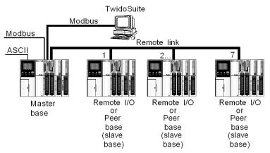
**NOTE:** Communication between the "Modbus" and "Remote Link" protocols cannot occur at the same time.
