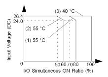
When using TWDLMDA40DUK and TWDLMDA40DTK limit the inputs and outputs, respectively, which turn on simultaneously along line (2).
