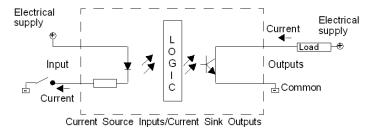
Input side COM field terminal connects to +24V field power supply. Output side COM field terminal connects to the "-" terminal or common of the field power supply.
