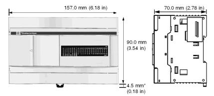
NOTE: \* 8.5 mm (0.33 in) when the clamp is pulled out.
