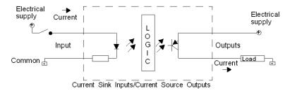
Input side COM field terminal connects to the "-" terminal or common of the field power supply. Output side COM field terminal connects to +24V field power supply.
