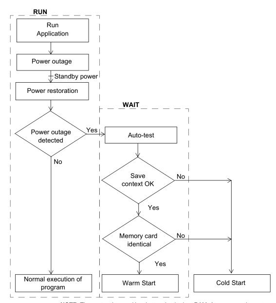
**NOTE:** The context is saved in a battery backed-up RAM. At power up, the system checks the state of the battery and the saved context to decide if a warm start can occur.
