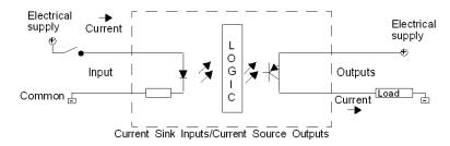
Input side COM field terminal connects to the "-" terminal or common of the field power supply. Output side COM field terminal connects to +24V field power supply.
