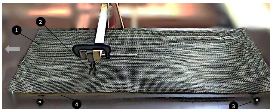
Fig. 2 . Designed laboratory facility photo: 1 - strainer mesh; 2 - fixed brush; 3 - frame
